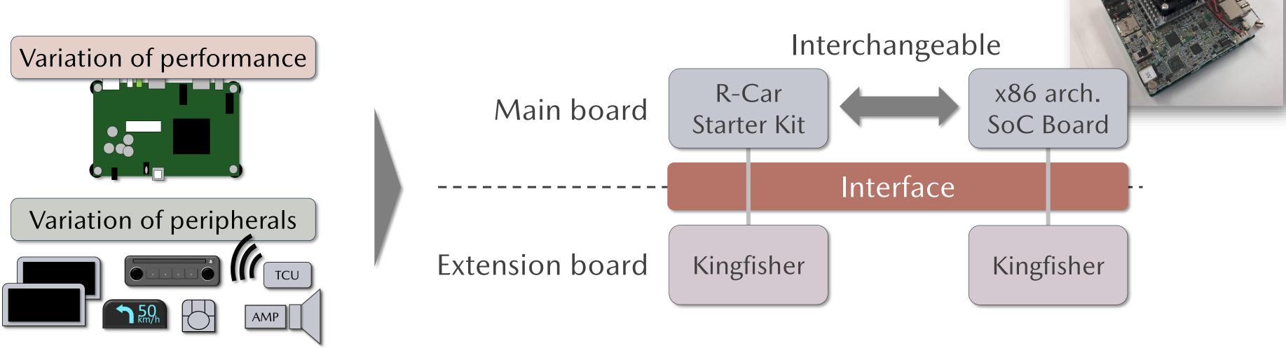
Developed x86 SoC board connectable to Kingfisher validated and verified the interchangeability with R-Car Starter Kit
